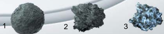
Tribodynamic activation (TDA) changes particle surfaces in a highly effective manner: 1: Result from classic milling; 2: result from an opposed jet mill; 3: Result from TDA
